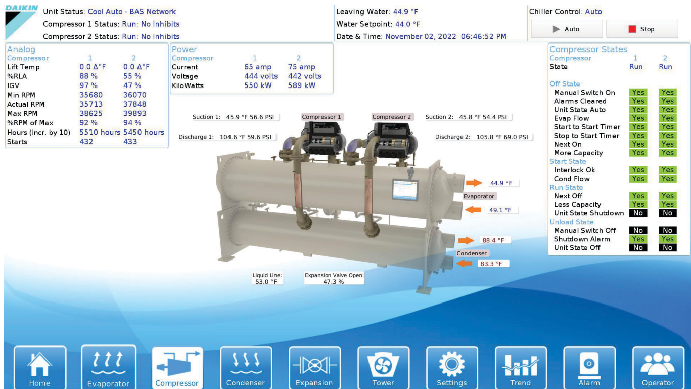
Figure 29: Compressor Details Information
