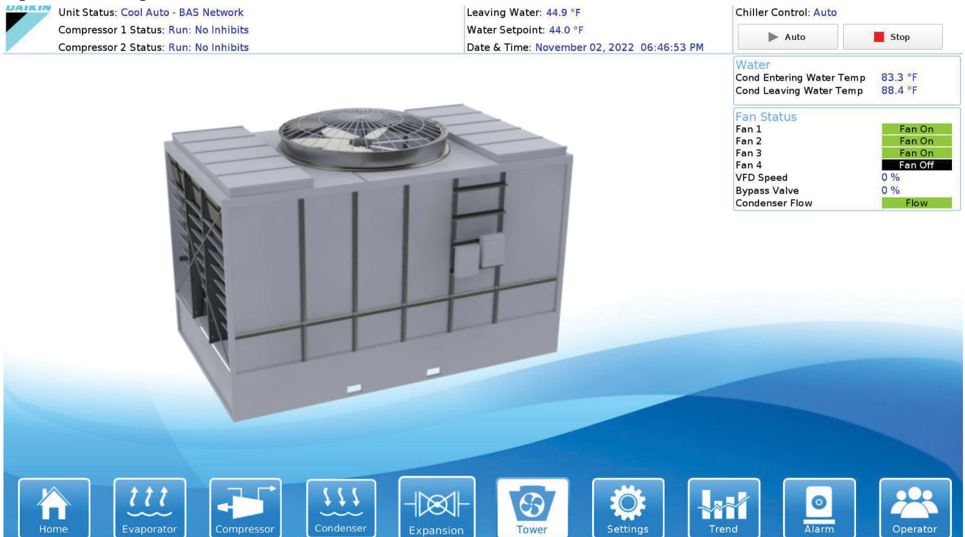
Figure 33: Cooling Tower Information
