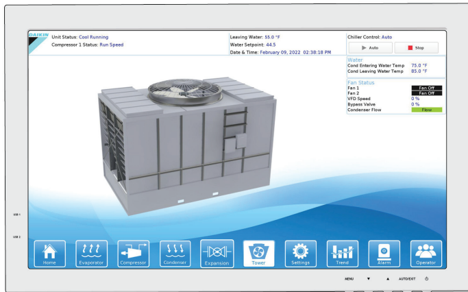
Figure 37: Cooling Tower Information
