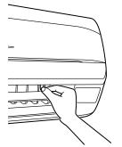
Stop the vertical flaps at a position where you can hold the tabs and adjust the louver left and right.
