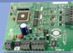
PC-100... Burglar alarm panel direct interface module
