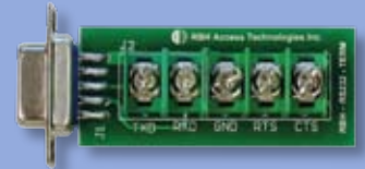
232-TERM... RS-232 DB9 adaptor with screw down terminals
