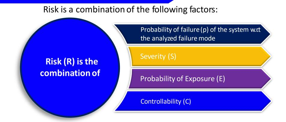
Hazard Analysis and Risk Assessment: evaluate **Potential Risk** of system in case of malfunction → "Thought Experiment" assuming that the failure mode is present (p = 1)
