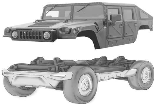
Fig. 6. Upper Body and Chassis of HMMWV.
