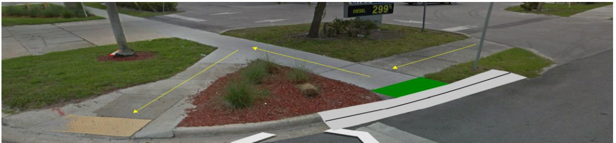
12.6.21 Minimum design changes are proposed for W. Delaware/Immokalee Rd. Currently, pedestrians have to zig-zag (see yellow arrows above), removal of sidewalks (green), add new sidewalk (grey/black dots), replace curb and drop curb (grey) for a more direct route to curb for pedestrians (yellow arrow below).
