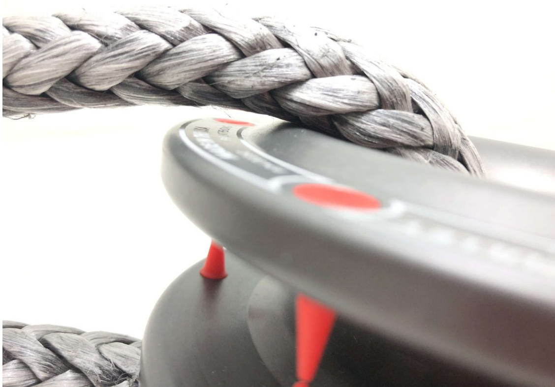
Photo 4 - Close Up of Soft Shackle Use & Positioning
