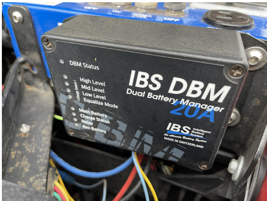
I mounted my IBS DC-to-DC charger in my engine bay, near my starter battery. Chargers will have multiple wires that need to be connected to a variety of cables under the engine hood.
