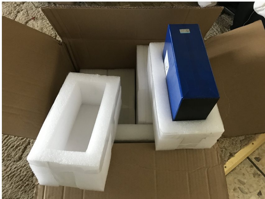
Pictured is the unboxing of one of my four purchased 3.2-volt, 280 AH LiFePO4 batteries. Four times 3.2 = 12.8 volts.
