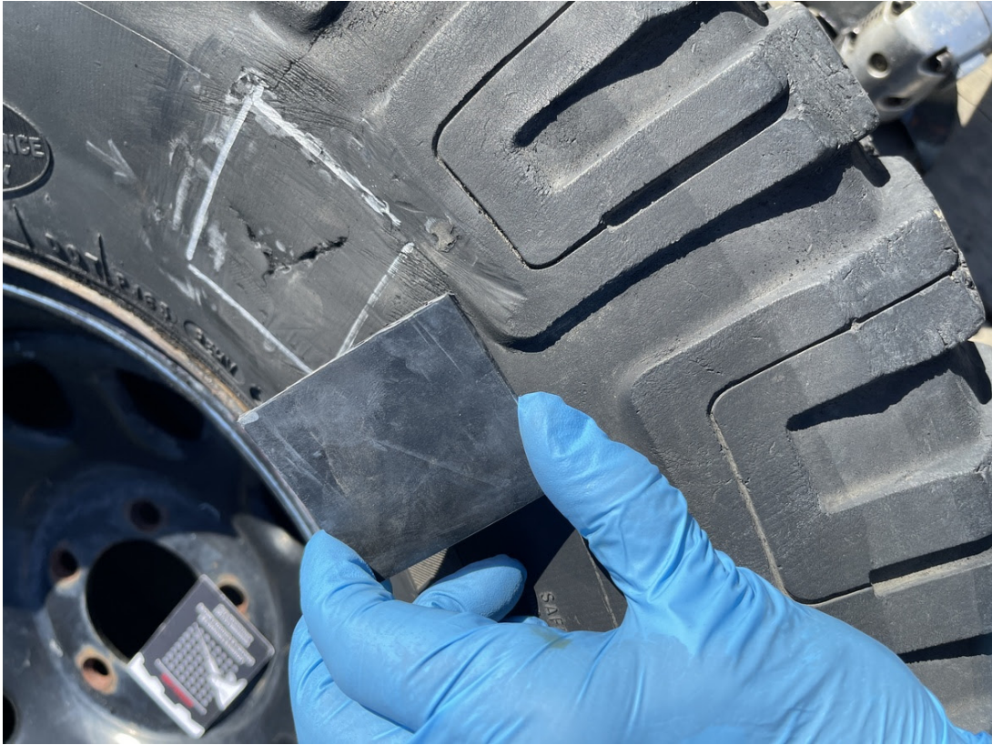
Getting a patch ready for gluing
