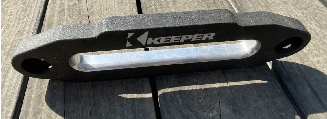
A poorly designed fairlead included with my Keeper winch.
