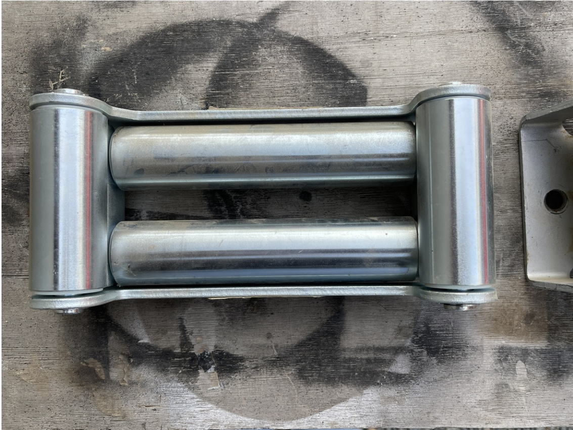
This new roller fairlead may be used with synthetic rope winch line.
