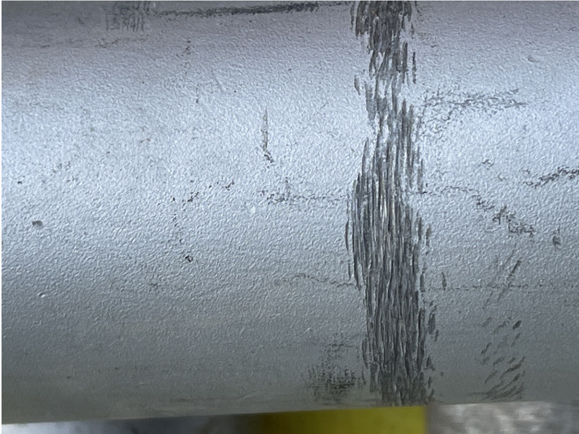
Fairlead metal roller with sharp scars capable of degrading synthetic rope winch line.
