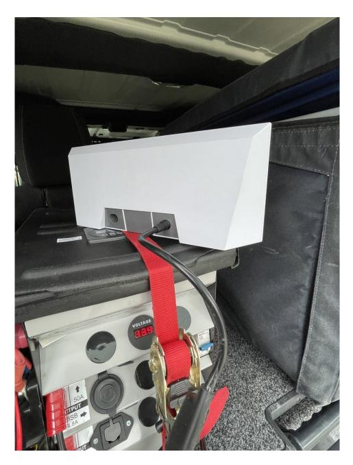
The Trio Power Supply is simply attached to your house battery on its "plus" and "negative" posts and then the unit's barrel connector seamlessly plugs into the Starlink's router.
