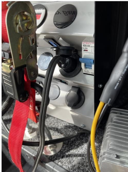
After connecting the Trio power supply I used my multimeter tester to measure the input and output of volts, then resistance (ohms). All the numbers were excellent so I went ahead connected the Starlink router and Gen 3 dish.
