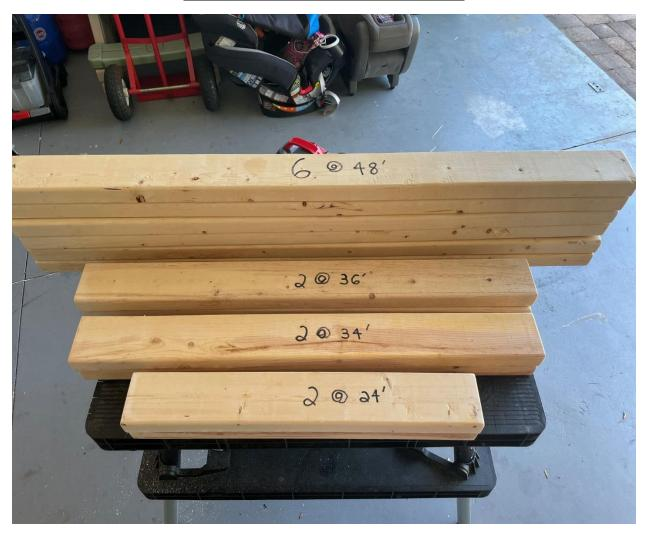
Required 5- 2 X 4s Cut to various lengths needed to build the Basic Trebuchet Base
