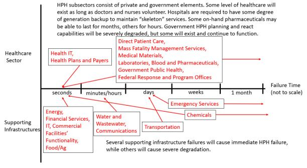
**Failure timeline:** (subsectors sourced from HPH SSP) Many aspects of the HPH sector will fail in seconds in a BSE. Other aspects of HPH will have a robust capability for hours as services are gradually curtailed.<sup>22</sup> Facilities will remain, but without power they will become less useful. Doctors and nurses can perform their duties "manually", but without modern facilities and equipment, their capability will be vastly reduced (if they continue to work at all). It is unclear
