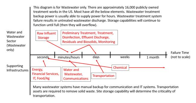
**Failure timeline**: Wastewater systems rely on gravity as sewage flows downhill. Pumps elevate sewage so that it may have a downhill flow for the next leg of its journey. If not pumped,
