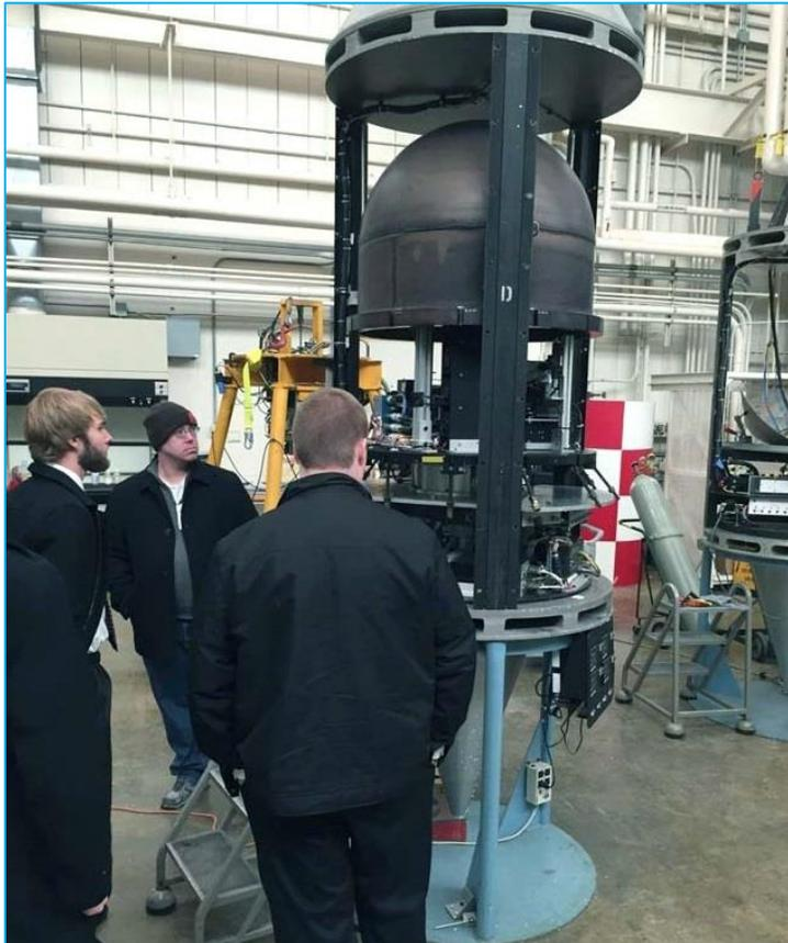
Examining a drop vehicle used to carry experiments and instrumentation during free fall experiments inside of a 467 ft. long vacuum chamber.
