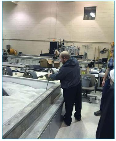
Demonstrating the consistency of the simulated lunar soil in the soil tank.
