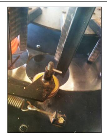
To return to singles trap: lift and rotate the pin (to the left) to rest in the slot.
