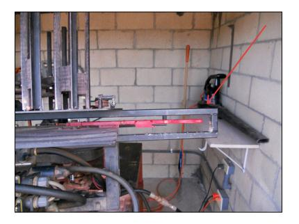
If the throwing arm is not in the (SAFE) position go to DE-COCKING procedures. Ensure no one is standing in front of the Trap Machine, and Ensure you are positioned below the throwing plate.
