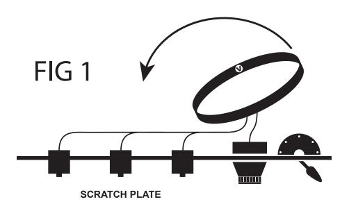
With the noise reduced mark the dot on the inner face of the NRS with an arrow pointing towards the scratch plate so as to be able to install the NRS module into the control cavity keeping the correct orientation of the NRS during final assembly.
