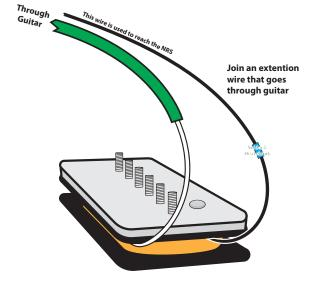
Add a length of wire (not supplied) to ground wire to pass through the guitar alongside the other pickup wire
