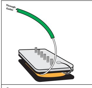
On back of p90 pickup de-solder ground wire (usually black) that is soldered to metal plate
