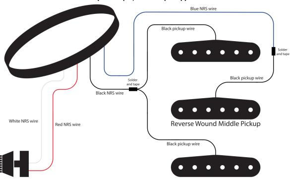
Solder wires to back of volume pot
