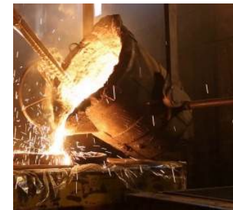
CASTING BY ELECTRIC INDUCTION FURNACE
