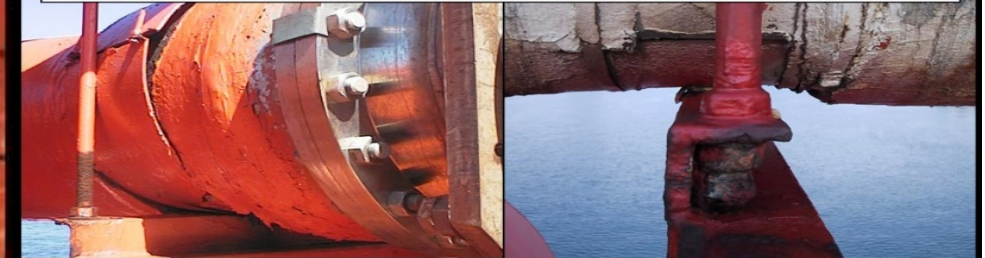
Crushed insulation material result in failure of Pipe support area Support Insulation areas are part of the pipes structural support. Ice Crushed insulation at those locations can cause very dangerous situations for pipe rupture caused by vibrations and friction to ships structure
