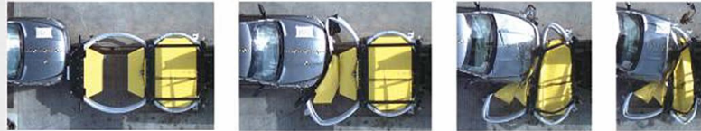
Scorpion II ® TL-3 TMA Impacted by 5,046 lbs (2,289 kg) Pick-Up Truck
