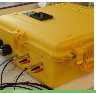
EcoCat-P instruments can provide two types of analysis and control, these are direct feedback monitoring and control of Gas Phase Composition or a calibrated continuous record of the entire gas phase.
