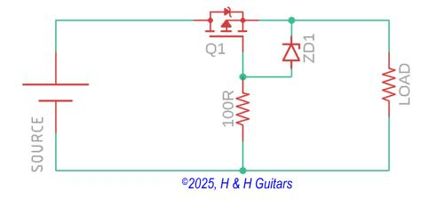
The P-MOSFET is a type of transistor that uses an electric field to control the flow of current through it. FETs are devices with three terminals that are source, gate, and drain. FETs control the flow of current by the application of a voltage to the gate, which in turn alters the conductivity between the drain and source. This is the basic principle that is incorporated in using a P-MOSFET as a switch in reverse polarity protection.
