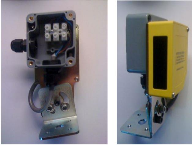
Verify Installation: Once the system is installed, POWER ON THE SENSORS AND CHECK THAT ALL RIDERS ARE PICKED UP (LED comes on). If needed the sensitivity range may be adjusted. (See manufacturer's instructions included). Sensing range is 8" to 80". Adjust the range so that the riders are picked up but not the water. There is a delay adjustment that we set before shipping, to eliminate splashing water from triggering the sensor.
