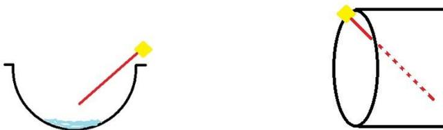
The entrance sensor should be mounted far enough down the slide so that a rider does not activate the sensor while waiting in the staging area. On a tube slide, the sensor can be mounted so that it points into the tube. They should also be mounted facing away from the prevailing angle of the sun because they are infra-red sensors. Sensors must be mounted at a slight angle to the water.
