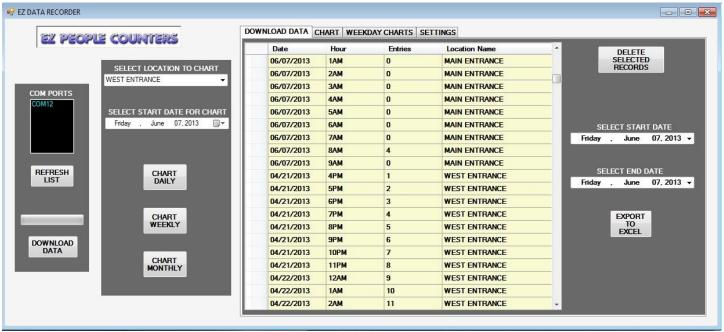
The "COM PORTS" will list the active USB/COM ports on your PC. If none are listed, make sure the USB cable is plugged in and click on the "REFRESH LIST" button. If more than one port is being used, you will be prompted to select the COM port, by clicking on the COM port in the list. If you do not know which port to select, do the following:
