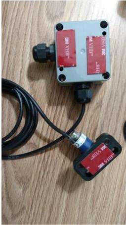
Verify Installation: Once the system is installed, POWER ON THE SENSORS AND CHECK THAT ALL RIDERS ARE PICKED UP (LED comes on). Sensing range is up to 13 feet.
