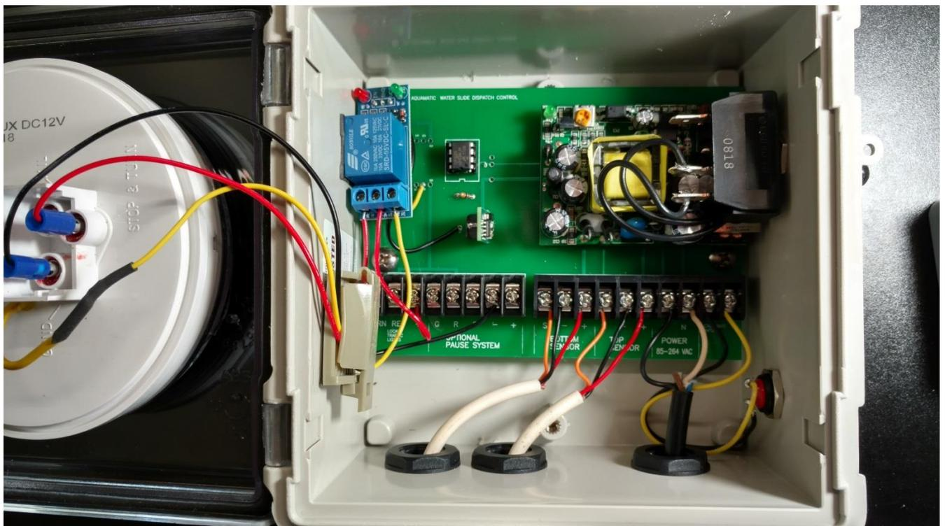
Mount the traffic light using the MOUNTING TABS (feet). All wiring cable glands or conduit must be run to the bottom of the enclosure.
