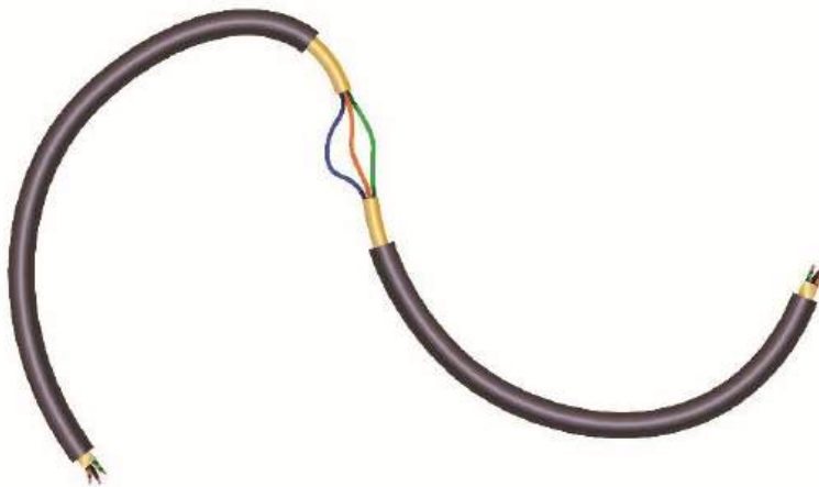
Example of exposed wiring on an electrical cord
