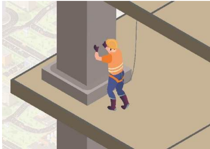
An example of a safe working area when using a Fall Arrest System
