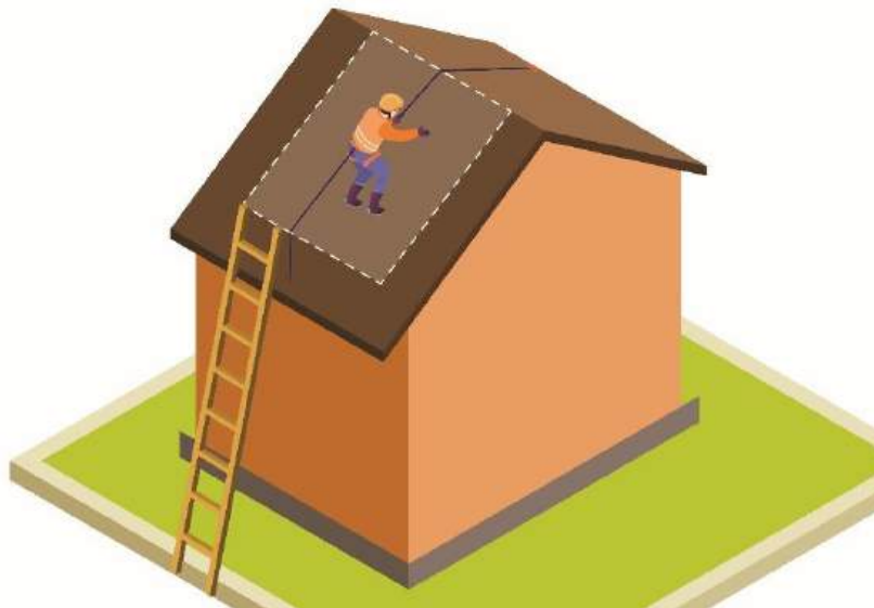
An example of a travel restraint system on a rooftop
