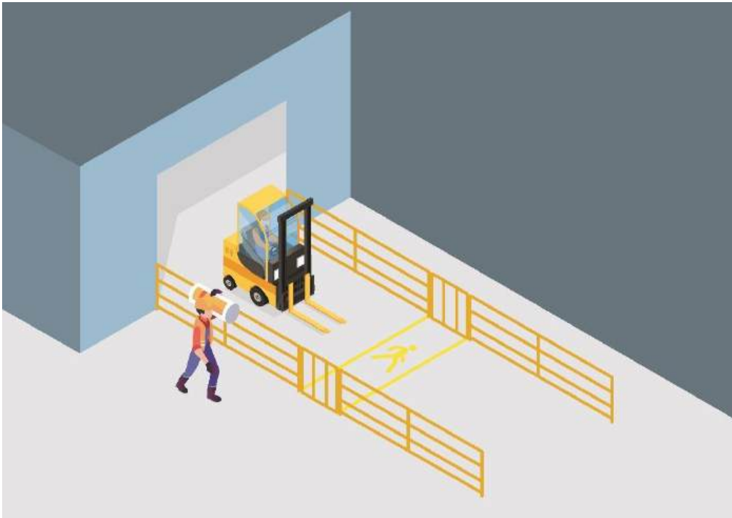
Guardrail at an exit
