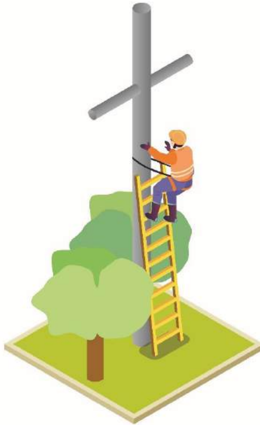
An example of a worker using a ladder and fall restraint system
