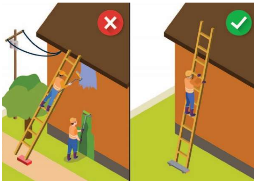
Examples of the correct and incorrect ladder setup and usage
