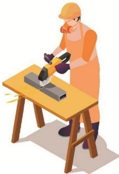
Example of wet cutting method and suitable PPE
