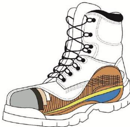
A cross section view of a safety boot with a toe cap
