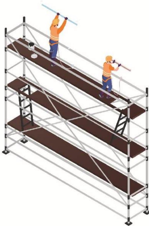
An example of scaffolding for personnel
