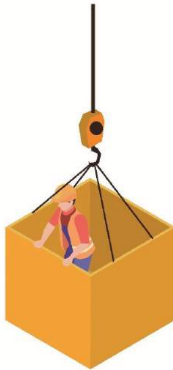
An example of a Work Box
