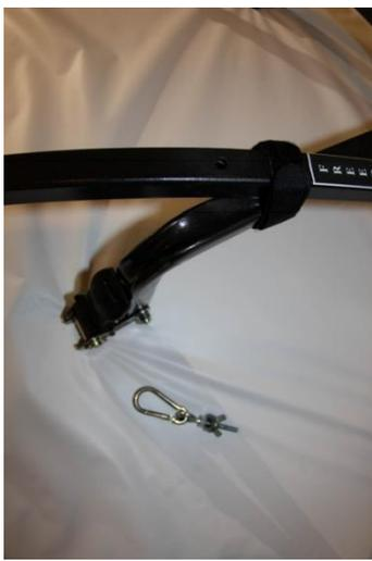
Once you've lined up the holes in the inner pole and the outer pole, secure one set of pole bolts. There will be two sets in your kit. Each set should consist of two eye bolts, two carabiners (snap links), three regular nuts, one wing nut, and 4 washers. Each set will have the two eye bolts attached by the carabiners with the nut, wing nut, and washers. Each eye bolt will have a regular nut snugged up against the eye. One will have an additional regular nut, the other will have a wing nut.
