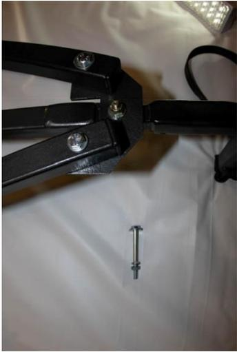
And...the longest of the bolts. This bolt replaces the center bolt on the lower bracket. The current bolt is designed for the lower leg and a flat piece of metal. The longer bolt accommodates the lower leg and an outer pole for use with the standard Freedom Flyer or a Triple Threat.
