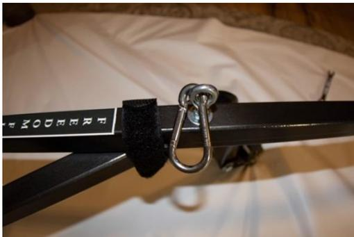
Once you've tightened the eye bolt, use the open end of the wrench to move the eye so that it is inline with the pole. This is the optimal position for attaching your flag and will help it flutter correctly.
