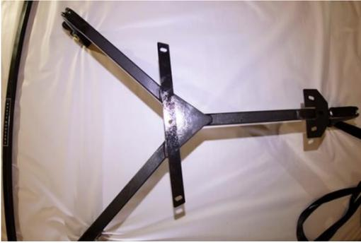
Next, place the upper bracket across the top portion of the triangle between the two upper arms of the Talon so that the holes are aligned. Ensure that the angled edges of the bracket are positioned as they are in the picture to the left.
