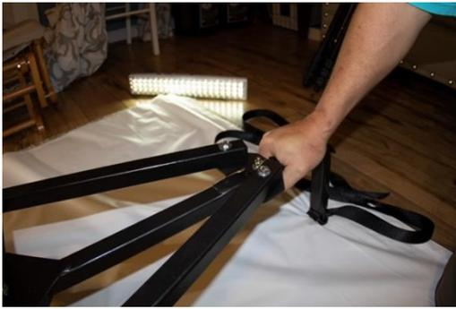
At this point, you will need one of the hands from your extra set to apply pressure to the lower leg to keep the unit from tipping as you insert the inner poles. If your extra set of hands has abandoned you, this can be accomplished with a dumbbell, the edge of a couch, or a large cat...as long as its lazy and you are fairly certain it won't become disinterested in helping and move halfway through the process.
