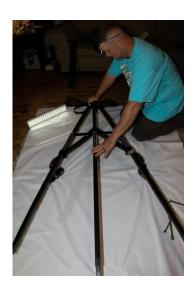
In order to install a third pole, simply remove the center bolts on both brackets, position a pole in the center, and reinstall the longer bolts.
