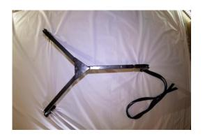
This piece is referred to as the "Talon"...prior to bolting anything together, take your talon out to your vehicle. The bottom foot is adjustable and will slide out without the bolt in it. Place the two upper arms (with ratchets attached) over the top of your tire. Slide the bottom arm in, paying close attention to which hole allows the bottom foot to be closest to the tire. It does not have to rest against the tire, you just want to make a mental not of the most snug fitting.
