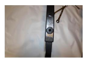
You will find that the hole at the top of the outer pole lines up with a hole on the inner pole. Insert the outer portion of the fastener through the holes pushing it down until the top is flush against the pole. At this point, your extra set of hands is probably kicked back with a cold beverage, giddy with excitement of the impending case of extreme patriotism in which they are about to participate.
