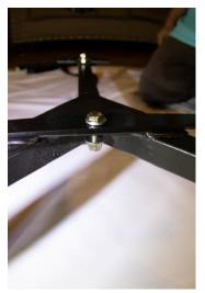
Next you will use the shorter bolt. This time, you are going to insert the bolt "down" through the bracket and then the hole in the triangle at the top of the Talon. For this bolt, there will be a washer on both sides. The lock nut is underneath and out of site. Again, DO NOT tighten this bolt all the way down at this time as it too will need to move around later in the instructions.
