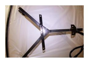
Next, place the upper bracket across the top portion of the triangle between the two upper arms of the Talon so that the holes are aligned. Ensure that the angled edges of the bracket are positioned as they are in the picture to the left.
