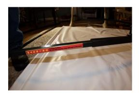
To install the inner pole, make sure that the warning label is facing the outside of the unit. This makes the label visible to anyone who may borrow your Double Threat when they extend the poles incase you forget to mention that the extended configuration should only be used when stationary, or at parade speeds less that 15 MPH.
