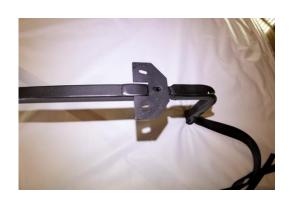
The "U" shaped bracket is positioned over the hole that is used to attach the bottom foot to the Talon. Notice there is a spacer welded to the lower arm of the Talon. The cut out portion of the "U" shaped bracket should but up against the spacer. They will not butt up against each other perfectly, and that's OK, as long as the holes line up.
