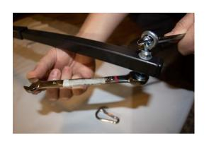
Next, take the other eye bolt from the first set (with the regular nut on it) and attach it to the top of the inner pole. With the eye on the same side of the pole as the lower eye bolt, insert the bolt through the top hole ensuring that one regular nut is tightened all the way against the eye. Install a washer on both sides of the pole. Attach the nut on the bottom side and tighten.
