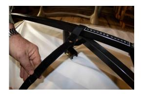
Placement should be just below the hole in the outer pole where the pole crosses over the upper arm of the talon.
