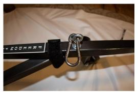
Once you've lined up the holes in the inner pole and the outer pole, secure one set of pole bolts. There will be two sets in your kit. Each set should consist of two eye bolts, two carabiners (snap links), three regular nuts, one wing nut, and 4 washers. Each set will have the two eye bolts attached by the carabiners with the nut, wing nut, and washers. Each eye bolt will have a regular nut snugged up against the eye. One will have an additional regular nut, the other will have a wing nut.
