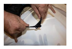
After tightening all the bolts, you will need the Velcro straps included in your kit. When you place the free running end of the strap through the buckle, it should "catch" on the Velcro. This indicates that you have it inserted correctly. Now that you know the direction you need to insert it, remove it from the buckle and wrap it around the outer pole AND the top arm of the Talon.
