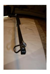
Once the nut is tightened on the back side of the inner pole, use the open end of your wrench to line the eye up with the pole. Repeat the steps for installing the inner pole on the other side.
