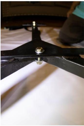
Next you will use the shorter bolt. This time, you are going to insert the bolt “down” through the bracket and then the hole in the triangle at the top of the Talon. For this bolt, there will be a washer on both sides. The lock nut is underneath and out of site. Again, DO NOT tighten this bolt all the way down at this time as it too will need to move around later in the instructions.
