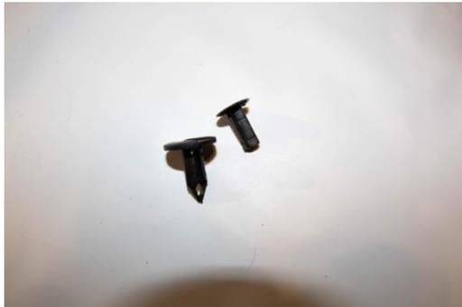
Also in your kit, you will find an optional plastic fastener. This is the last step so you're almost there! If you've ever removed a plastic piece from a Jeep Wrangler, you are familiar with these fasteners. The easiest way is to remove the center of the fastener so that it is in two pieces. If you are familiar with these, you may not need to separate them to accomplish this task.
