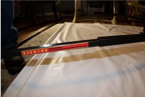
To install the inner pole, make sure that the warning label is facing the outside of the unit. This makes the label visible to anyone who may borrow your Double Threat when they extend the poles in case you forget to mention that the extended configuration should only be used when stationary, or at parade speeds less than 15 MPH.
