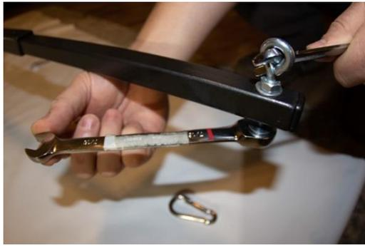
Next, take the other eye bolt from the first set (with the regular nut on it) and attach it to the top of the inner pole. With the eye on the same side of the pole as the lower eye bolt, insert the bolt through the top hole ensuring that one regular nut is tightened all the way against the eye. Install a washer on both sides of the pole. Attach the nut on the bottom side and tighten.
