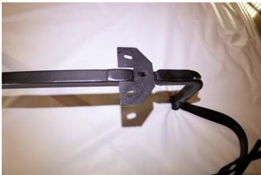
The "U" shaped bracket is positioned over the hole that is used to attach the bottom foot to the Talon. Notice there is a spacer welded to the lower arm of the Talon. The cut out portion of the "U" shaped bracket should butt up against the spacer. They will not butt up against each other perfectly, and that's OK, as long as the holes line up.
