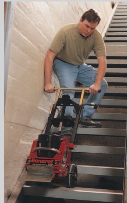
Wheels positioned for transporting up and down stairways.
