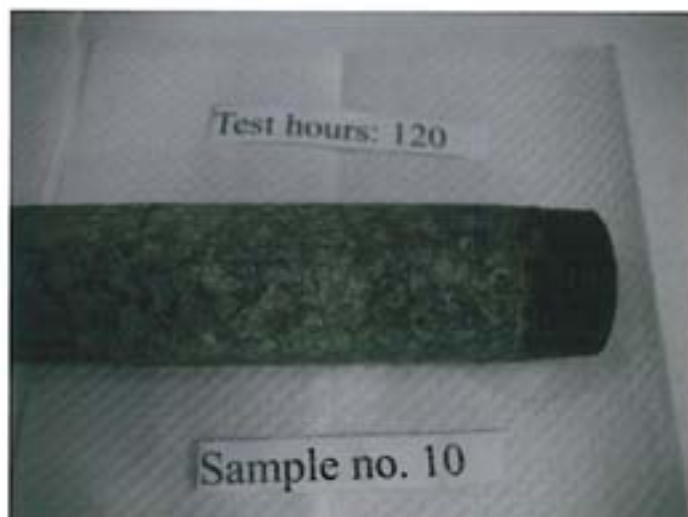
Sample After Testing – 120 hours (Sample 10)
