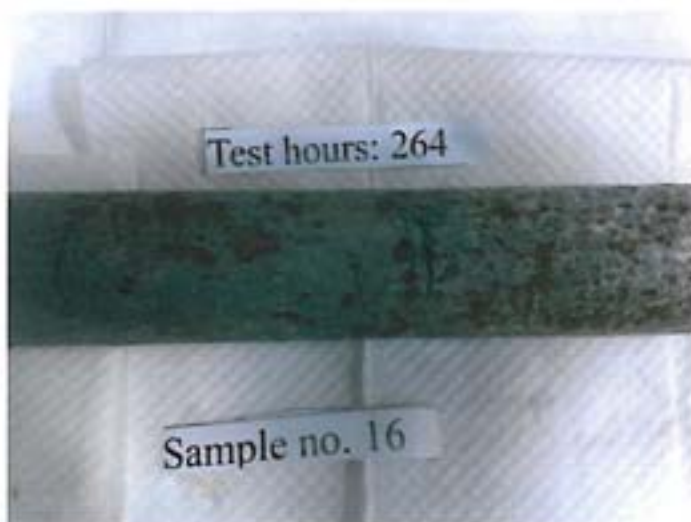
Sample After Testing – 264 hours (Sample 16-2)
