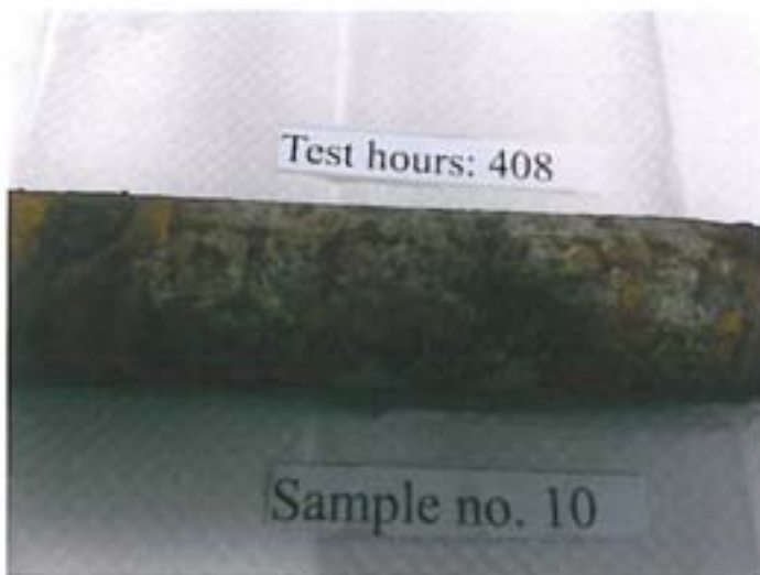
Sample After Testing – 408 hours (Sample 10)
