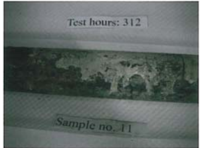
Sample After Testing – 312 hours (Sample 11)
