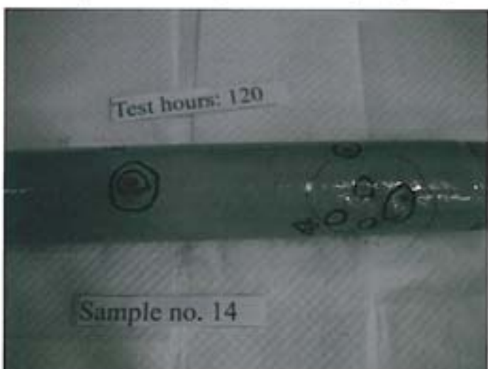
Sample After Testing – 120 hours (Sample 14)
