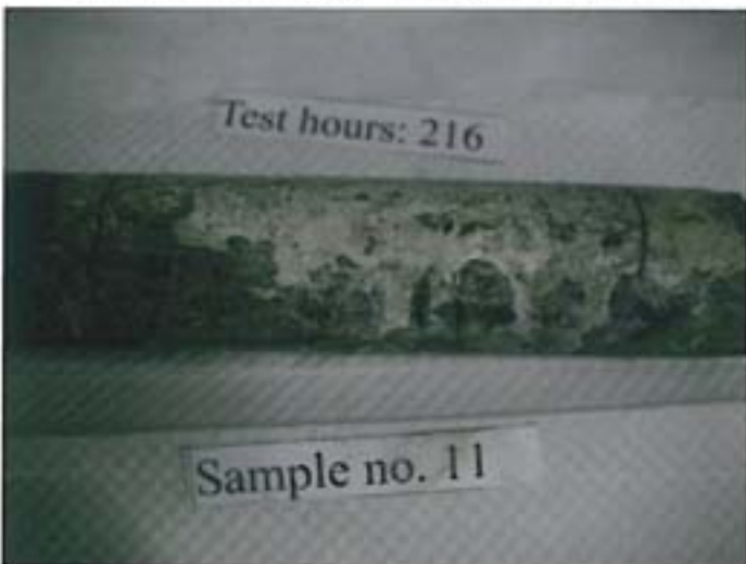
Sample After Testing – 216 hours (Sample 11)
