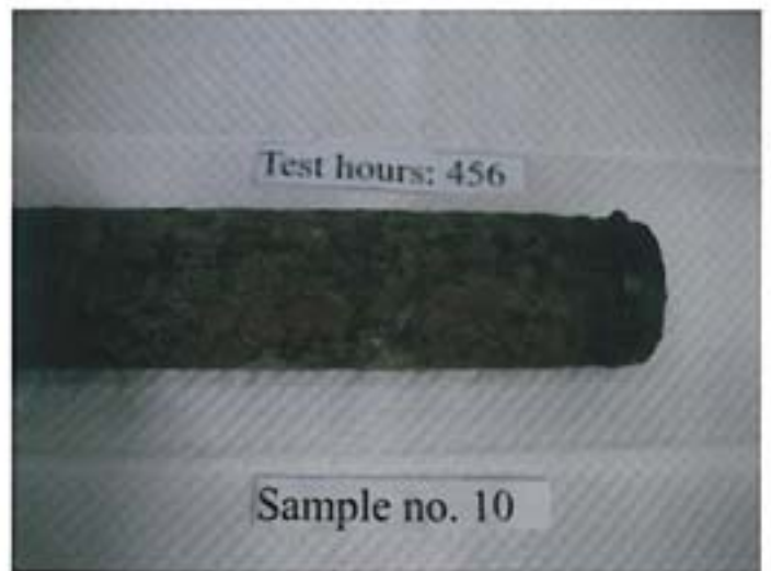
Sample After Testing – 456 hours (Sample 10)
