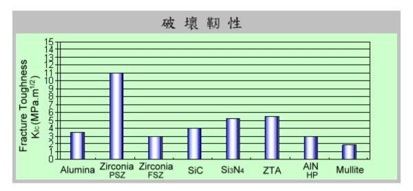
Only two types of PSZ & TZP (Tetragonal Zirconia Polycrystal, 90% tetragonal phase, add yttria) can supply highly strength & toughness, it mainly applies in the structural components which are requested wear-resisting & highly mechanical strength. At room temperature, its wear rate is higher about 3~5 times than Alumina. But, the mechanical strength is lowered at high temperature; for this
