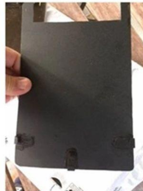
Here is the flap by itself. Notice that I epoxied on some metal flashing clips that I painted black. These stabilize
