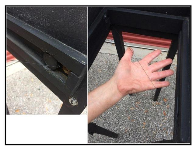
The photo on the left is the outside of the rope. It is wrapped with red plastic tape and goes through a narrow hole. Both sides have narrow holes. When the rope up pulled apart the two ends are stopped from coming out by the narrowness of the holes and the bulk of the magnets inside them.
