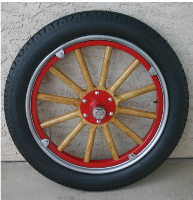
The black Firestone tires on the galvanize-colored rims mounted on the red felloes with the Golden Oak stained Hickory spokes and red hubs with nickel hubcaps are a beautiful array of colors on the artillery wheels for the Connecticut-Copperthite Pie Wagon.
