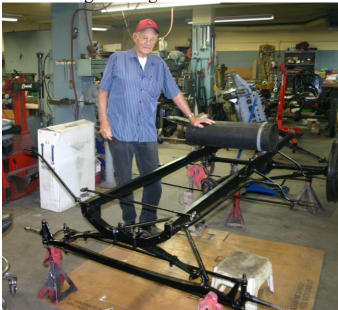
Here Gary is checking the oval fuel tank for proper fit to the frame.
