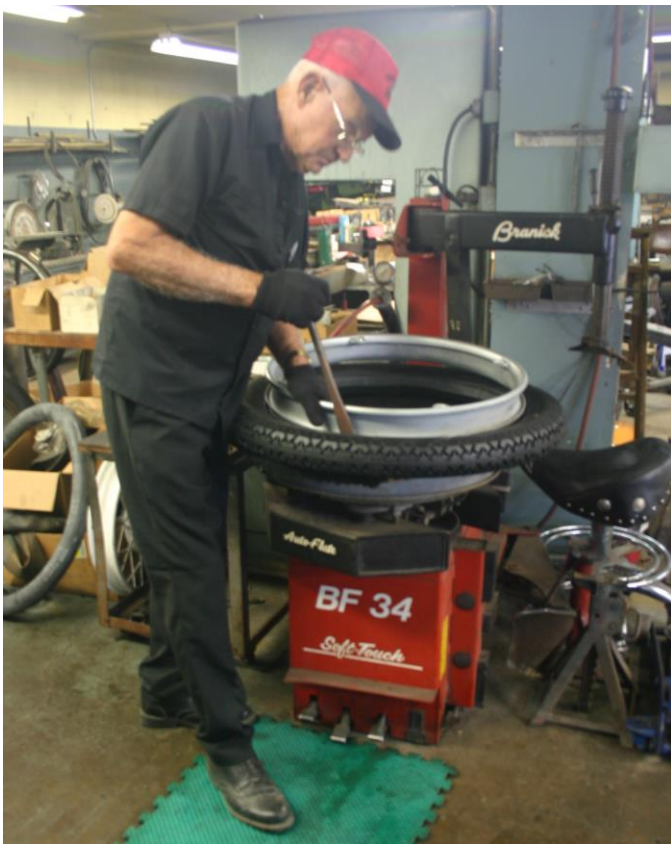
Gary Cooper delicately installs the new Firestone clincher tires (being very careful not to pinch the tubes) onto the demountable clincher rims for the Pie Wagon.
