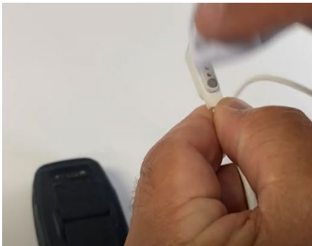
Clean the charger cable pins (very lightly) to remove dust and accumulated dirt.
