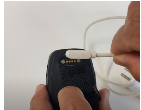
Cleaning the pins regularly helps to maintain a good charging contact and prolongs your device lifespan.
