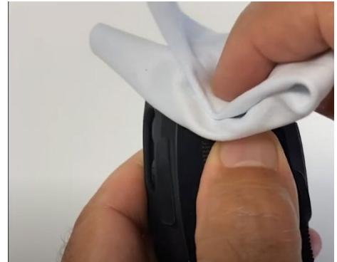
Clean the back contact pins with a soft cloth in order to remove dust and accumulated dirt.
