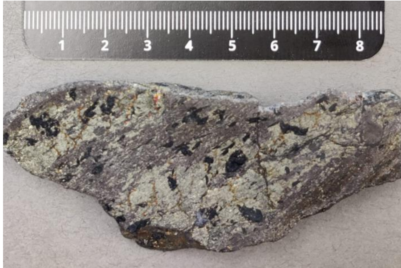
Float sample from River Ayr with 0.08ppm gold, 38ppm silver, 9.1% copper, 0.135% cobalt and 0.16% Zn
