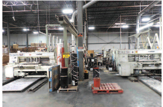
R&R has two Curioni mini 28-inch by 80-inch flexos running side by side and recently added a diecut section to one.
