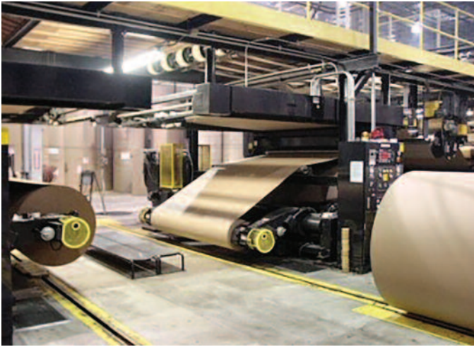
One of two Isowa heavy-duty corrugators at NewCorr Packaging in Northborough, Massachusetts, which provides several grades of board to R&R and other box makers in the Northeast.
