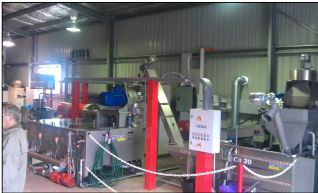
Top left: Olive press at left, twigs, leaves / olive separator and olive washer at right.
