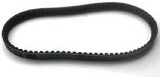
CVT (transmission) belt. Price ~ $40. Belt life anywhere from 2500 to 10,000 miles
