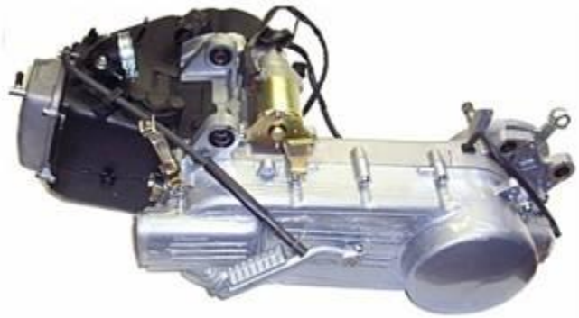
150cc engine and transmission as used in many Chinese scooters
