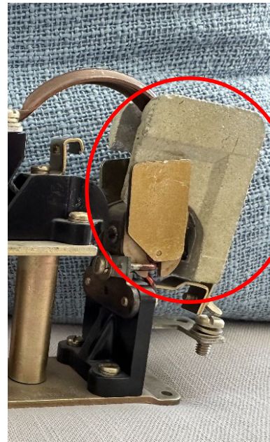
Photo #2 – Close up of Arc Chute
