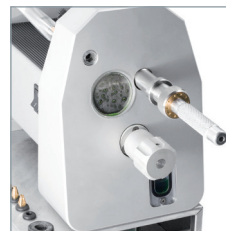
Cut the electrode by turning the handle.
