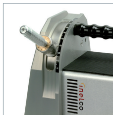
Grind the electrode in the desired angle.
