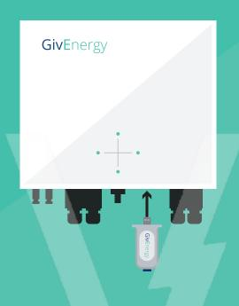
IMPORTANT! Please ensure the dongle is screwed into the bottom of the inverter on both sides.
