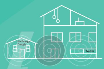
When installing the Inverter into an outbuilding, such as a garage, the signal may not be strong enough to reach the dongle.
