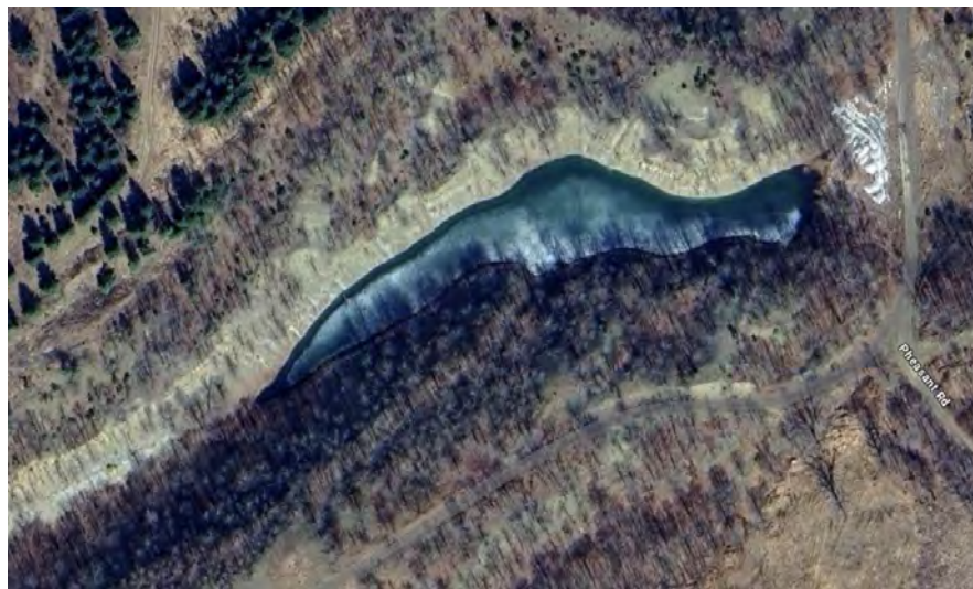
This image is an aerial view of the flooded strip mine cut. Water seeps through the road fill on the right side of the image.
