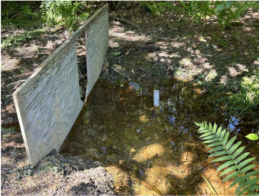
Weir and Transducer for MC2 During Low Flow Conditions
