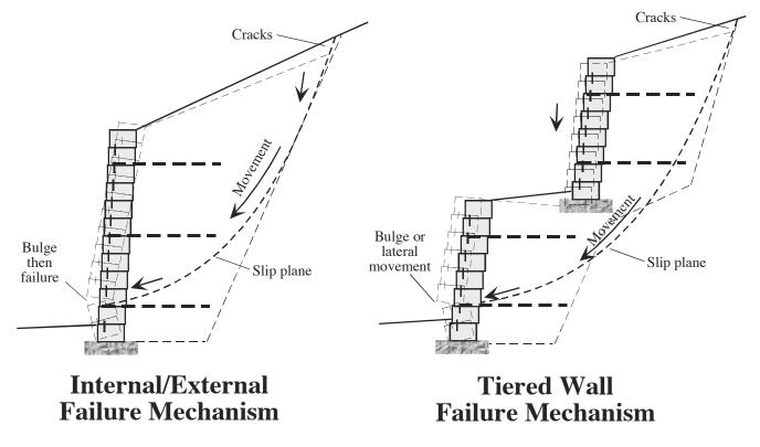
Reinforced walls are considerably more complex than simple gravity walls and must be designed accordingly. The soil strength and stability component of the design takes on much greater importance as the structures become taller requiring more attention to site specific soils information, proper design considerations, and contractor quality assurance provisions.
